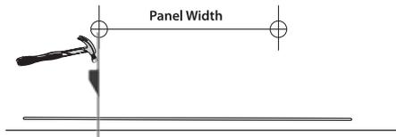
Hammer first stake into ground, aligned to string line. Stake fin tops should be at ground level.
