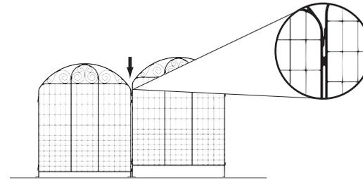
Insert and link together with installed panel.
