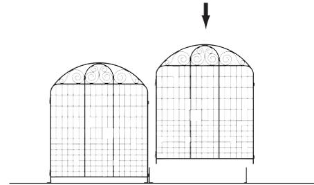
Position the next panel to mark the next stake placement in the soil.
