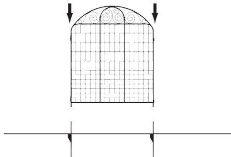
Place panel over stakes and insert onto the stakes.
