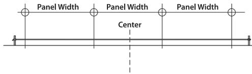
Stretch line along desired fence path. Determine starting point, usually a corner or the fence center.
