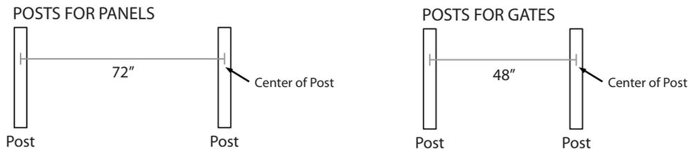
Layout the perimeter of determined fencing area with stakes and masons string to keep posts in line when installing. Place the wood stakes where you intend on installing the posts.
